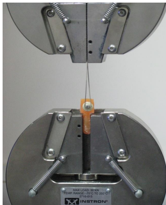
Fig: 1 Instron / Universal testing machine model no 3366 (instron corporation.) Shear bond strength testing
