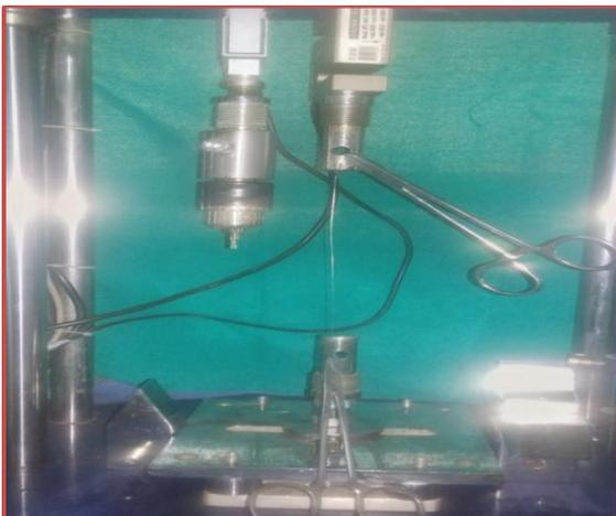
**Fig. 2: Shows stretching of stainless steel wire under tensile stretching forces at a uniform rate of 20mm/minute in Universal Testing Machine (UTM)**
