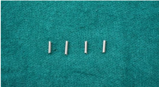
Fig 2: Steel tubes cut to the required length
